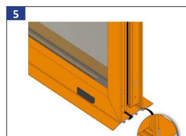
Install the first window in the continuous bead of sealant and use the snap trim clips provided.
