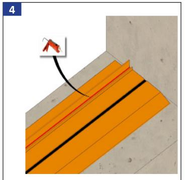
Apply a continuous bead of sealant into the track where the inside window leg will rest.
