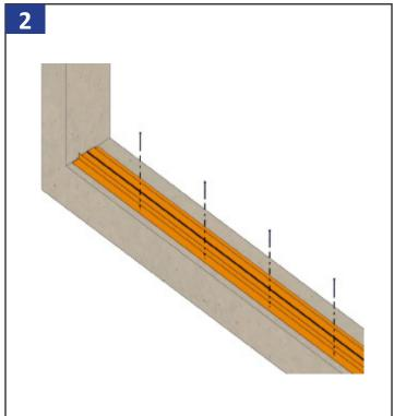
Set sill flasing on the continuous bed of sealant. Install through the interior anchor leg using fasteners supplied by the insaller.
