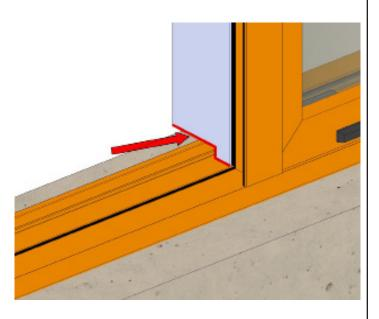
Cut T-Mull to match window height and notch at the sill (1/2  $\times$  2 3/4) to clear the interior leg of the sill flashing.
